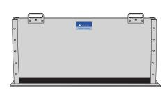
Inserting Shield: With label facing out, insert the bottom of plate into channels. Lower the shield until there is a firm and even connection with the sill. Tighten the tension screws.
