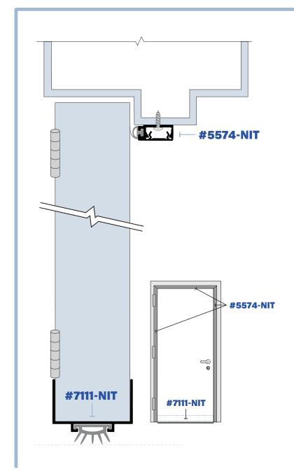
Nitrile rubber is a versatile addition to Legacy's arsenal of formulations for practical sealing solutions. Among its many benefits, nitrile rubber provides good compression set and tensile strength, and is resistant to heat, abrasion and moisture. Its resistance to gas permeability also makes it corrosion-resistant to a long list of chemicals.
