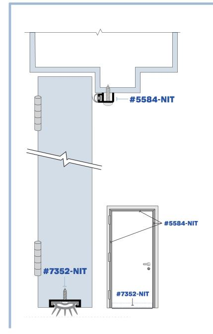
Nitrile rubber is a versatile addition to Legacy's arsenal of formulations for practical sealing solutions. Among its many benefits, nitrile rubber provides good compression set and tensile strength, and is resistant to heat, abrasion and moisture. Its resistance to gas permeability also makes it corrosion-resistant to a long list of chemicals.
